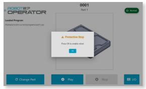
Operator can display when the UR robot goes into protective stop, and the user is able to clear the error from the interface.
