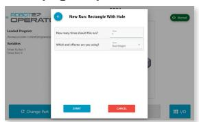
How many pieces, length, width, or any other needed variables can be set by the operator before the run.
